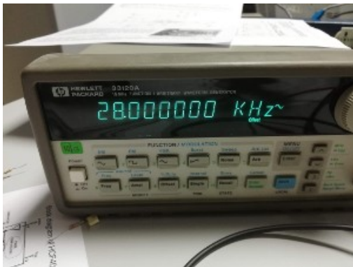
Sine generator Amplitude=4.5V; Frequency=28KHz
