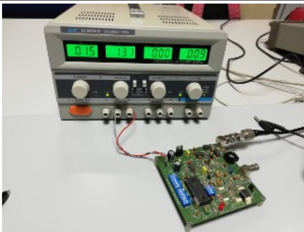
FM Transmitter Output Power=200mW
