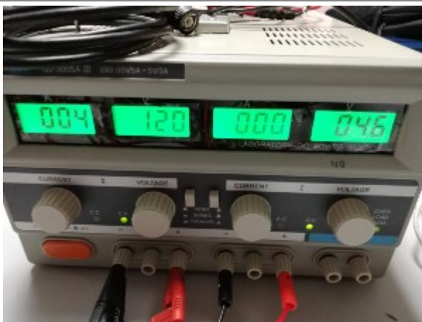
Power supply V_{cc}=12V ; V_{contr}=4,6V
