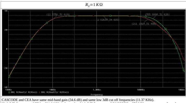
High 3dB frequency of CEA = 211,2 MHz is lower than high 3dB frequency of CASCODE = 356 MHz, as you expect from theory.
