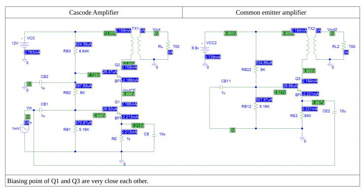
As it was done in point 2) plot the harmonic response of two amplifiers in the same plot. Identify and compare midband voltage gains, lower and upper 3dB cutoff frequencies of the two amplifiers.
