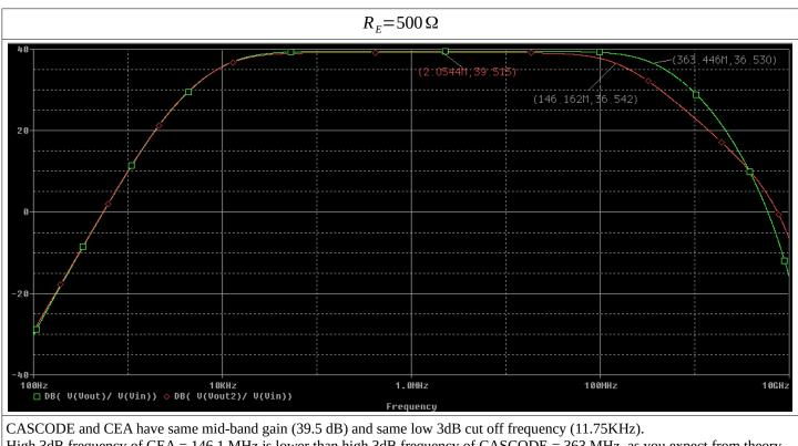
High 3dB frequency of CEA = 146.1 MHz is lower than high 3dB frequency of CASCODE = 363 MHz, as you expect from theory.
