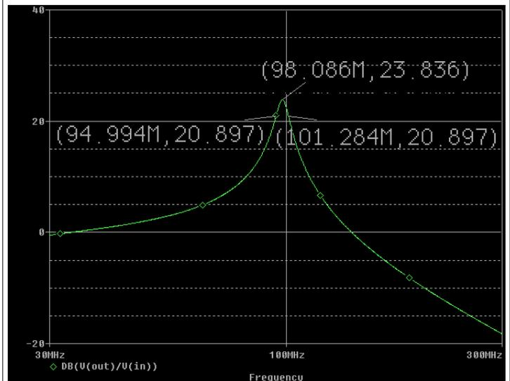
Maximum gain 23,84 dB at 98,086 MHz, Bandwidth 6,2 MHz, Q=15,82
