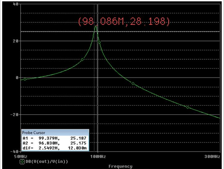
Maximum gain 28,2 dB at 98,086 MHz, Bandwidth 2.55 MHz, Q=38,46
