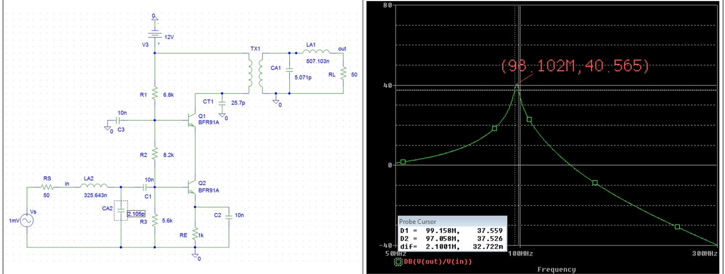
Maximum gain 40,56 dB at 98,102 MHz, Bandwidth 2,1 MHz, Q=46,72
