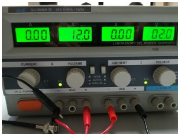
Power supply V_{cc}=12 V; V_{contr}=2,0 V
