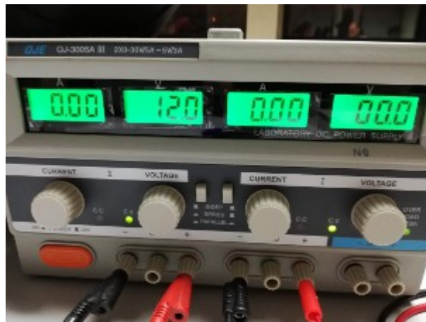
Power supply V_{cc}=12V ; V_{contr}=0V
