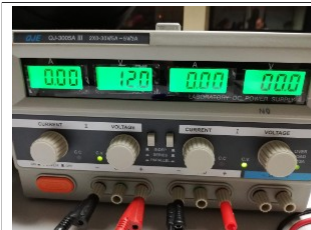
Power supply V_{cc}=12V ; V_{contr}=0V
