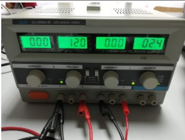
Power supply Vcc=12 V; Vcontr=2,4V
