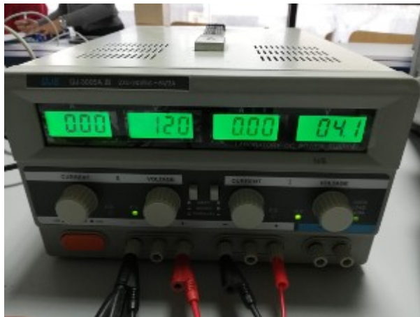
Power supply Vcc=12 V; Vcontr=4,1V
