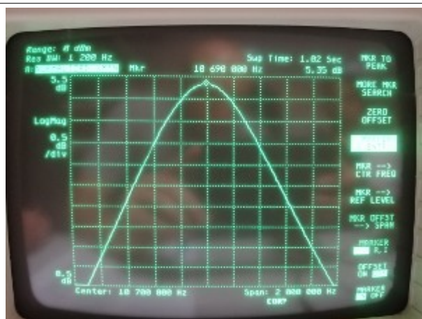
Network analyzer Center Frequency = 10,7 MHz; Span = 2 MHz
