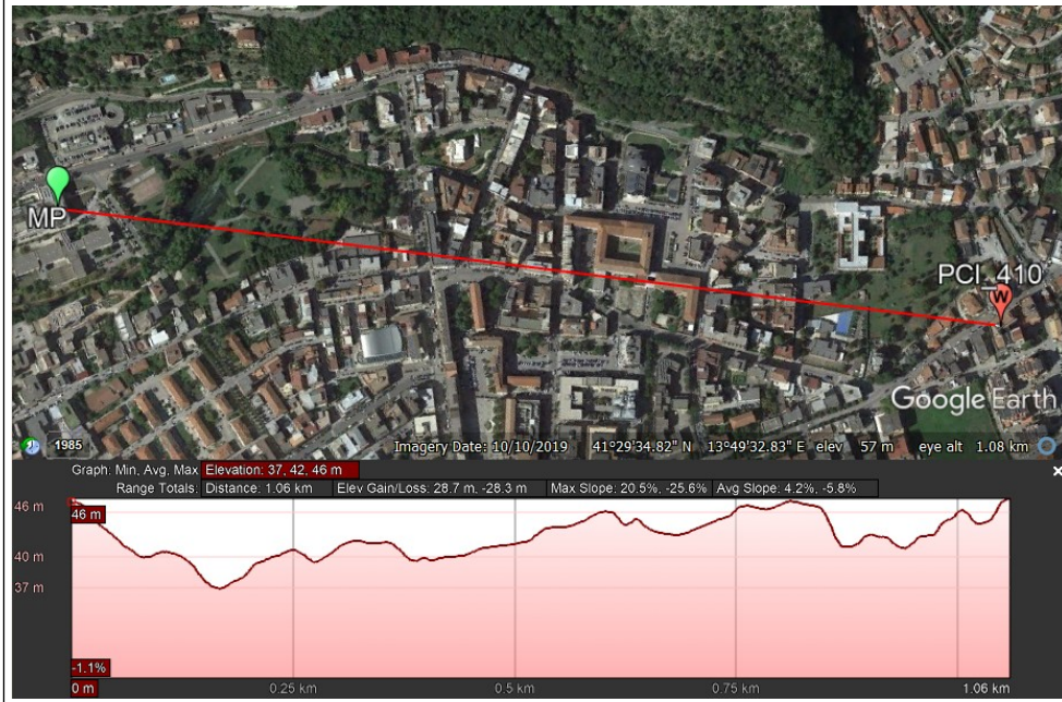
Figure 80: Google Earth [92] elevation profile from measurement point to base station cell PCI 410.
