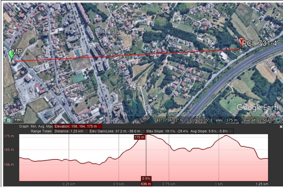
Figure 95: Google Earth [92] elevation profile from measurement point to base station cell PCI 731.
